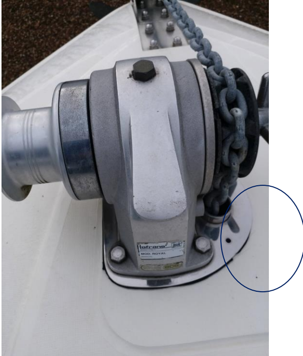
Fig 2. xxxxxx xxxxxxxx windlass with high moisture readings indicated by blue circular outline.
